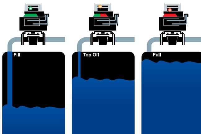
The Expeditor enables three position control of On/Off valves in combination with two standard solenoid valves.
