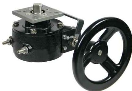
The RD Declutchable Gear Override enables manual operation of pneumatic actuated valves. The heavy-duty construction and water proof housing make the RD series suitable for installation in a wide range of environments and hazardous area applications.
