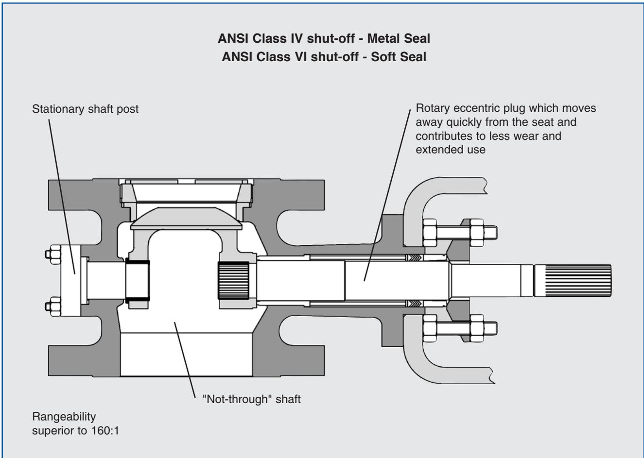
Figure 1: OpExc Rotary Plug Control Valve
