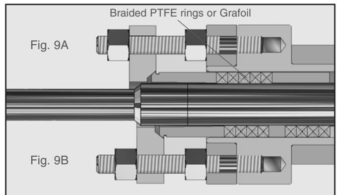
**Figure 9A: Packing: Formed Rings**
