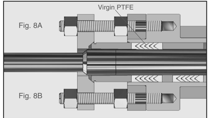
**Figure 8A: Standard Packing: “V” rings**
