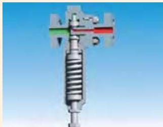
**Type C4 Fig 3 – Self Acting High Pressure PRV**
