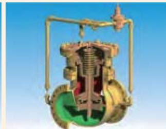
**Type WR – Pilot Operated High Capacity PRV**
